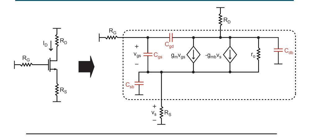
$$\begin{split} &C_{gs} = C_{gc} + C_{ov} = \frac{2}{3} C_{ox} W(L-2L_D) + C_{ov} \\ &C_{gd} = C_{ov} \\ &C_{sb} = C_{jsb} \quad \text{(area + perimeter junction capacitance)} \\ &C_{db} = C_{jdb} \quad \text{(area + perimeter junction capacitance)} \end{split}$$
