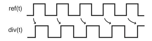
Resulting ramp in phase causes PD characteristic to be swept across its different regions (cycle slipping)
