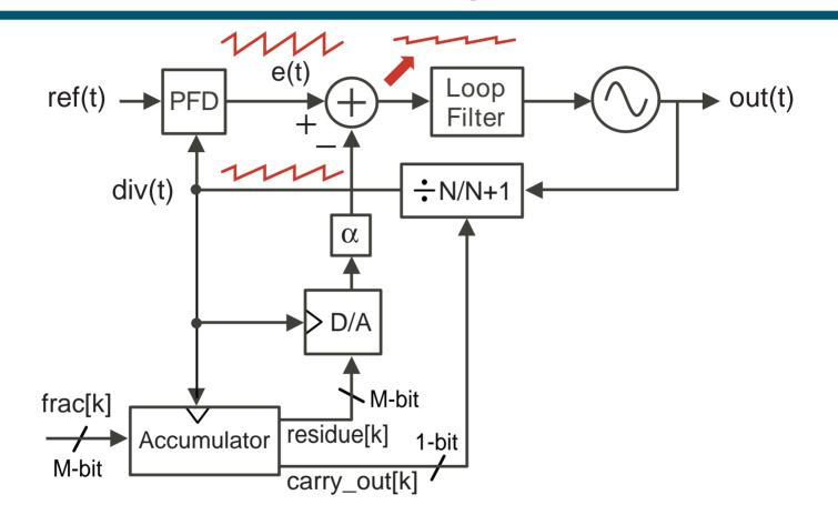
Gain matching between PFD error and scaled D/A output must be extremely precise
