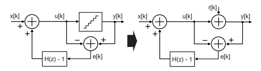
Represent quantizer block as a summing junction in which r[k] represents quantization error
