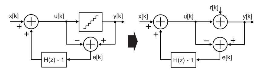
Calculate using Z-transform of signals in linearized model Y(z) = U(z) + R(z)
