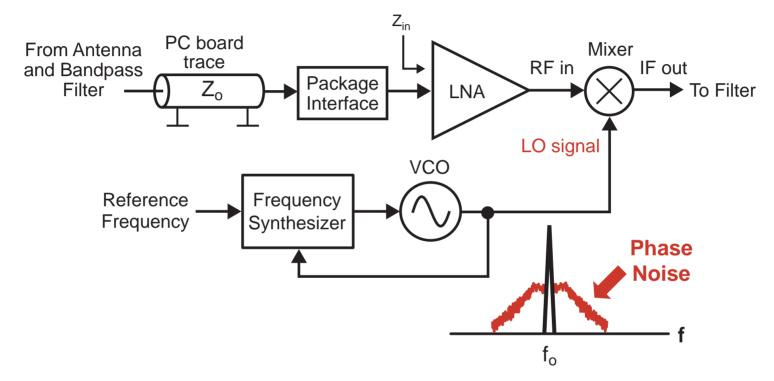
Synthesizer noise has a negative impact on system
