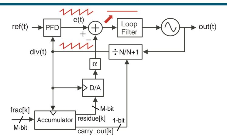
Phase error due to fractional technique is predicted by the instantaneous residue of the accumulator
