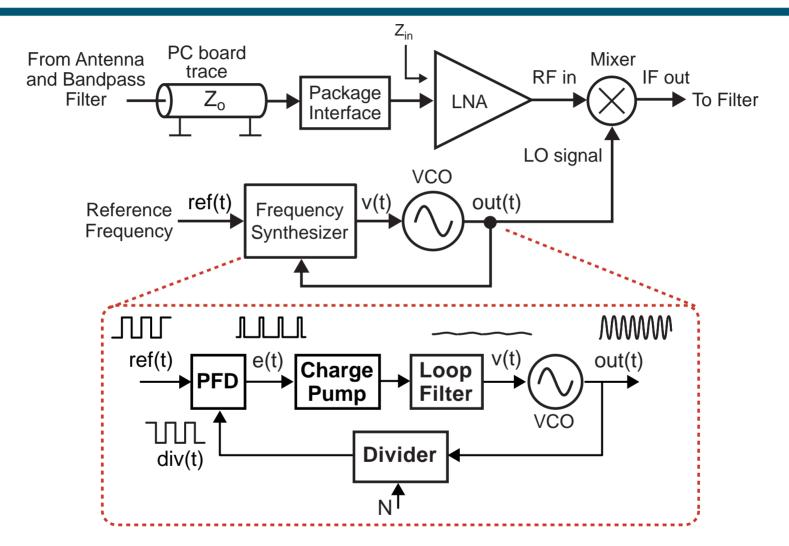
Design Issues: low noise, fast settling time, low power M.H. Perrott
