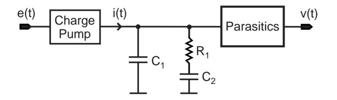
Example: include two parasitic poles with the lead/lag transfer function
