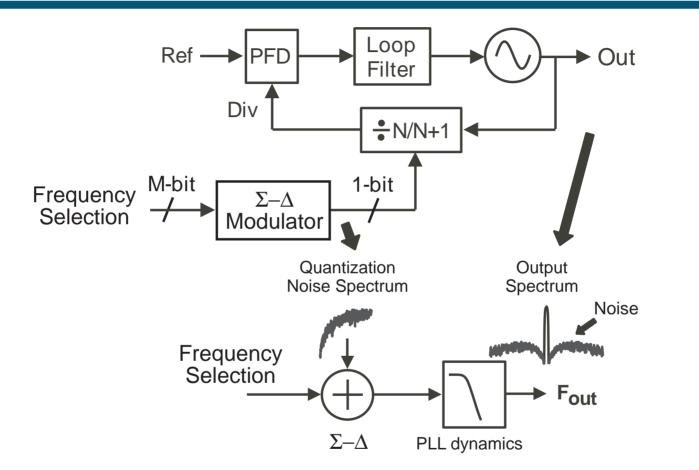
Lowpass action of PLL dynamics suppresses the shaped Σ-Δ quantization noise
