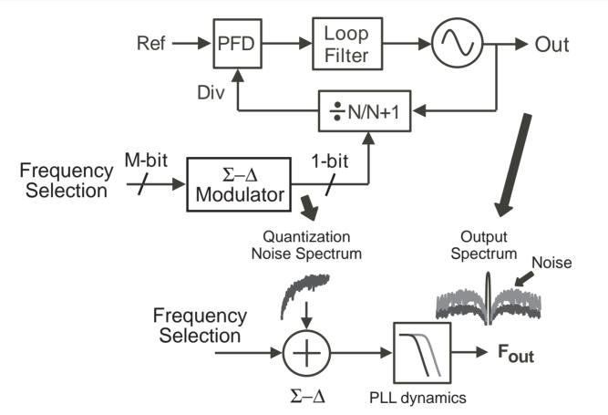
Higher PLL bandwidth leads to less quantization noise suppression
