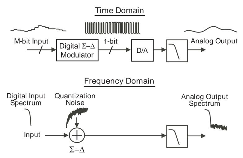
Sigma-Delta dithers in a manner such that resulting quantization noise is "shaped" to high frequencies
