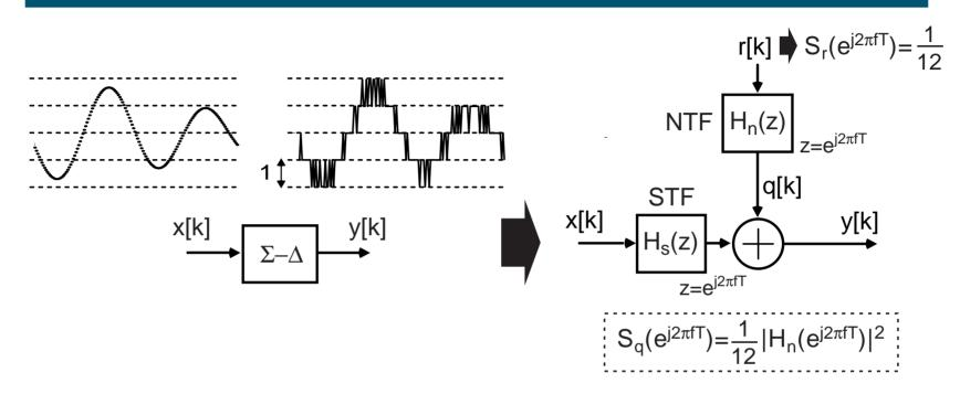
Composed of two transfer functions relating input and noise to output
