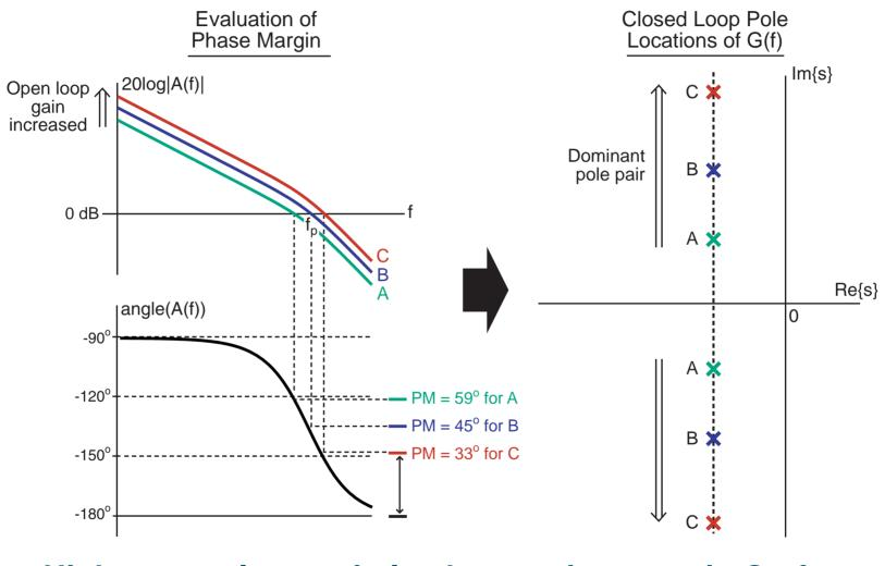
Higher open loop gain leads to an increase in Q of closed loop poles
