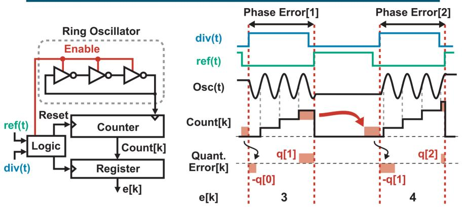
Enable ring oscillator only during measurement intervals
