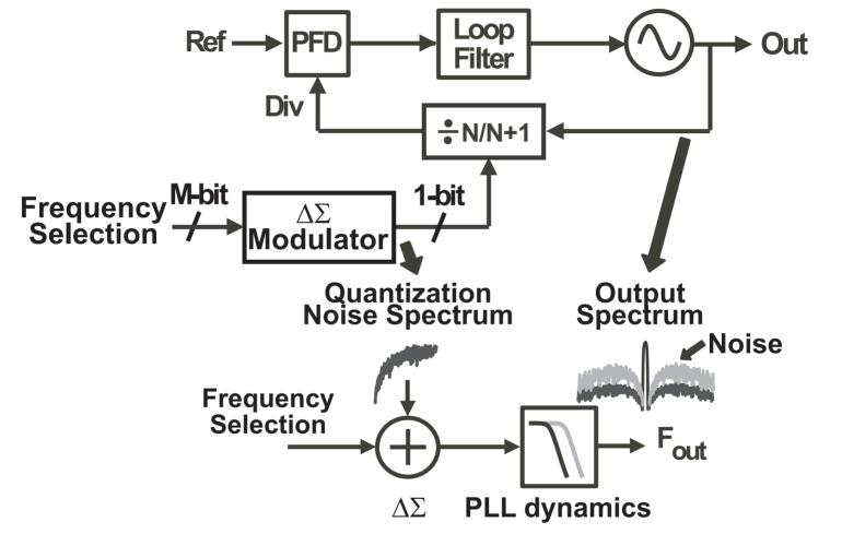
• Increasing PLL bandwidth increases impact of  $\Delta\Sigma$  fractional-N noise
