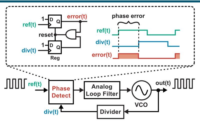
Pulse width is formed according to phase difference between two signals
