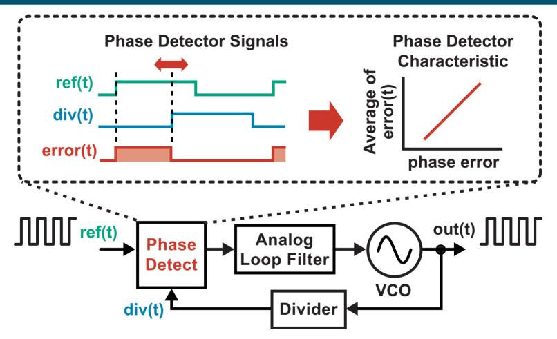
Benefit: average of pulsed output is a continuous, linear function of phase error
