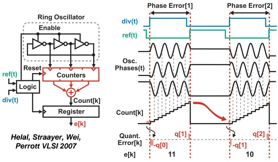
Raw resolution is set by inverter delay
