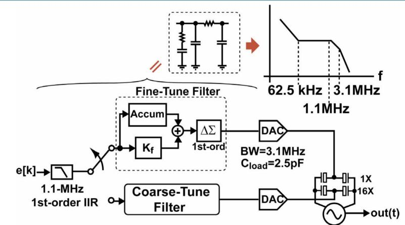
Equivalent to an analog lead-lag filter
