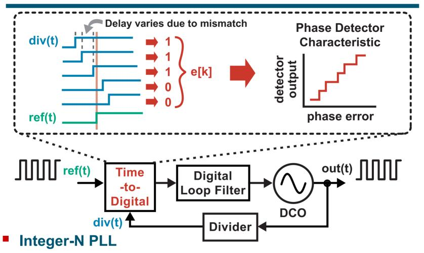
Limit cycles due to limited resolution (unless high ref noise)
