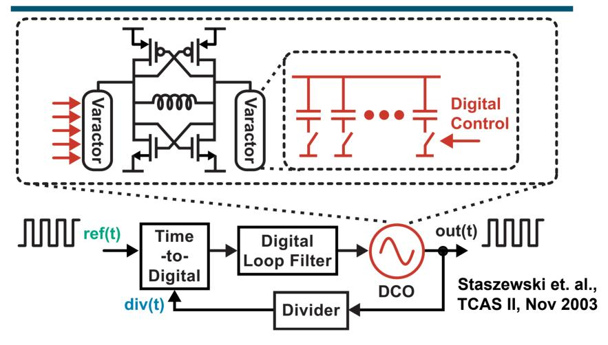
Adjust frequency in an LC oscillator by switching in a variable number of small capacitors
