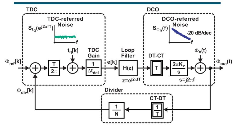
TDC and DCO-referred noise influence overall phase noise according to associated transfer functions to output
