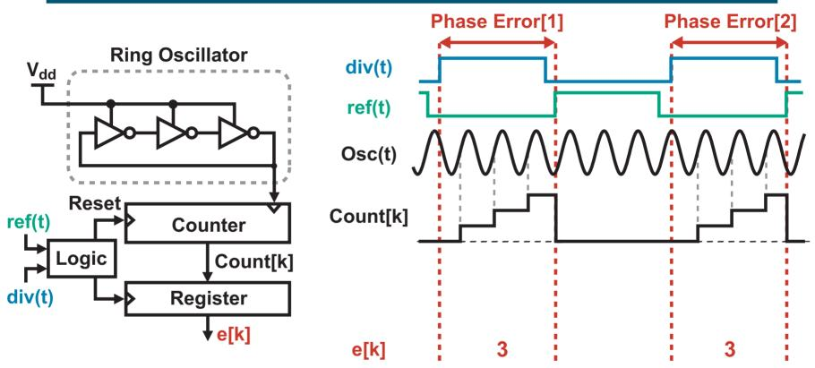
Output e[k] corresponds to the number of oscillator edges that occur during the measurement time window
